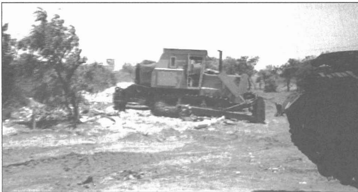
Figure 2. This Pakistani D7 bulldozer is equipped with a ripper fitted with MCAP. While used to clear roadblocks in Mogadishu, it is also well suited for locating firing wires.
