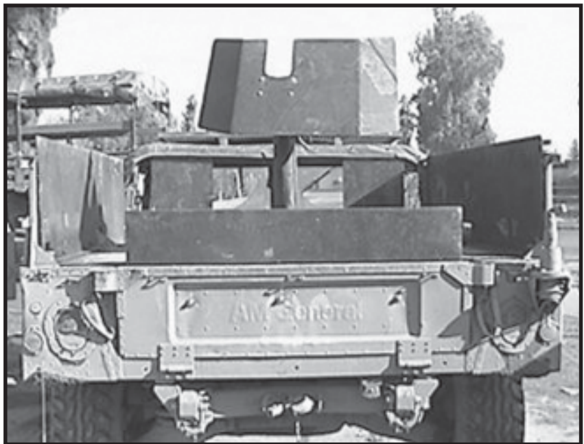
A HMMWV with a steel ballistic shield
