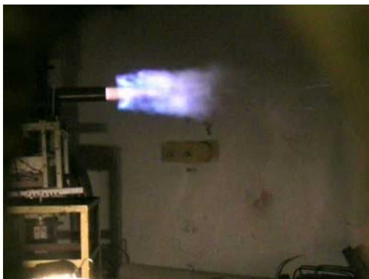
Figure 34: The plume of the predetonator operating on aviation kerosene – air mixture.
