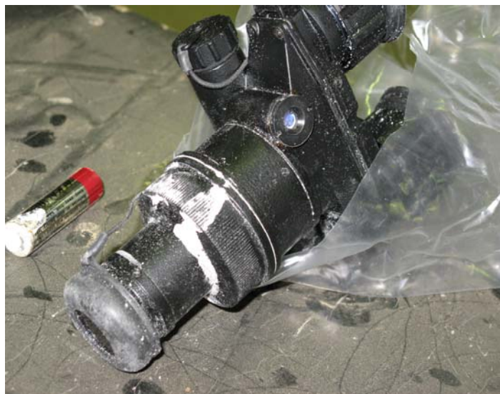
Figure 5: NVD Damaged by Leaking Battery
