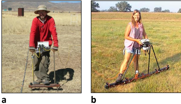
Figure 2. Commonly used resistance instruments and configurations: (a) TR/CIA resistance meter using .50-m twin probe array; (b) Geoscan RM-15 with MPX multiplexer using .50-m twin probe array.
