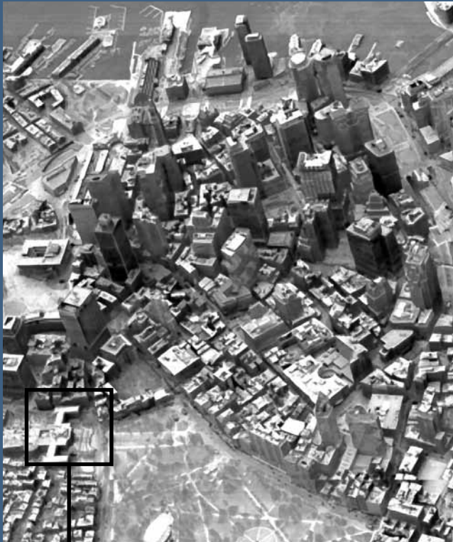
Aerial, winter night, infrared image of downtown Boston collected by a camera using the digital focal-plane array. The inset image of the Massachusetts State House partially illustrates the detail present in the image. Infrared image resolution is less than 1 meter, and the image quality is better than a high-definition television image.
