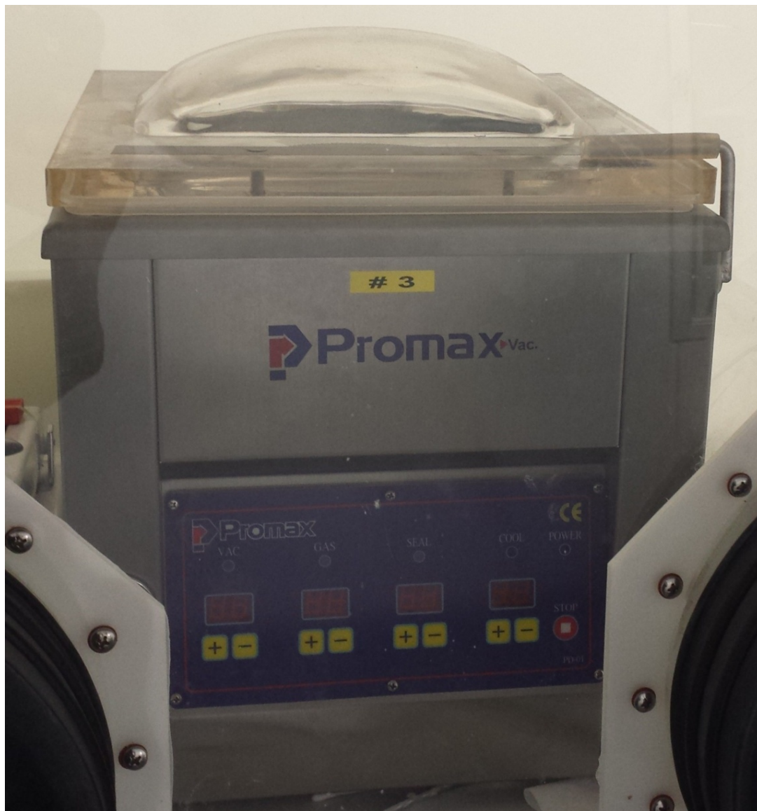
FIGURE 11: VACUUM HEAT SEALER FOR VACUUM RESEALING OF POUCHES
