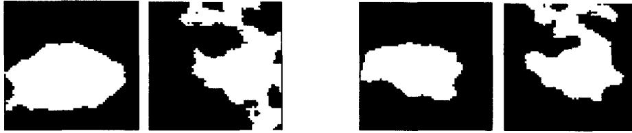
Scanned images of anti-tank mines Scanned images of anti-personnel mines (In each case, a good image is at left, and a bad image with narrow "bridges" is at right)
