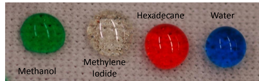
After dip-coating with a solution of fluorodecyl POSS
