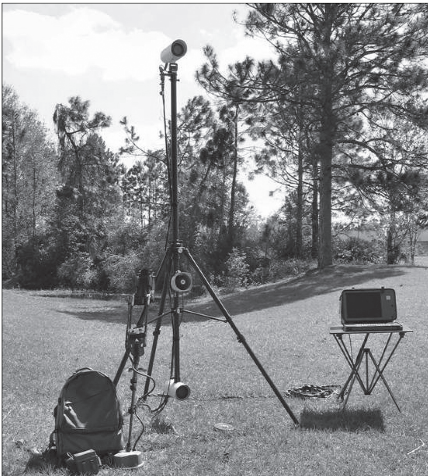
The Sweep Monitoring System (SMS) is a training aide that provides Soldiers with immediate feedback on their sweep techniques.
