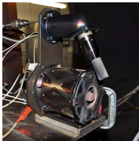
Fig. 1 Iodine Thruster in Test Facility
