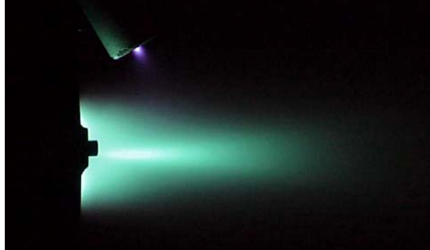
Fig. 5 Iodine Plume from 200 V Discharge
