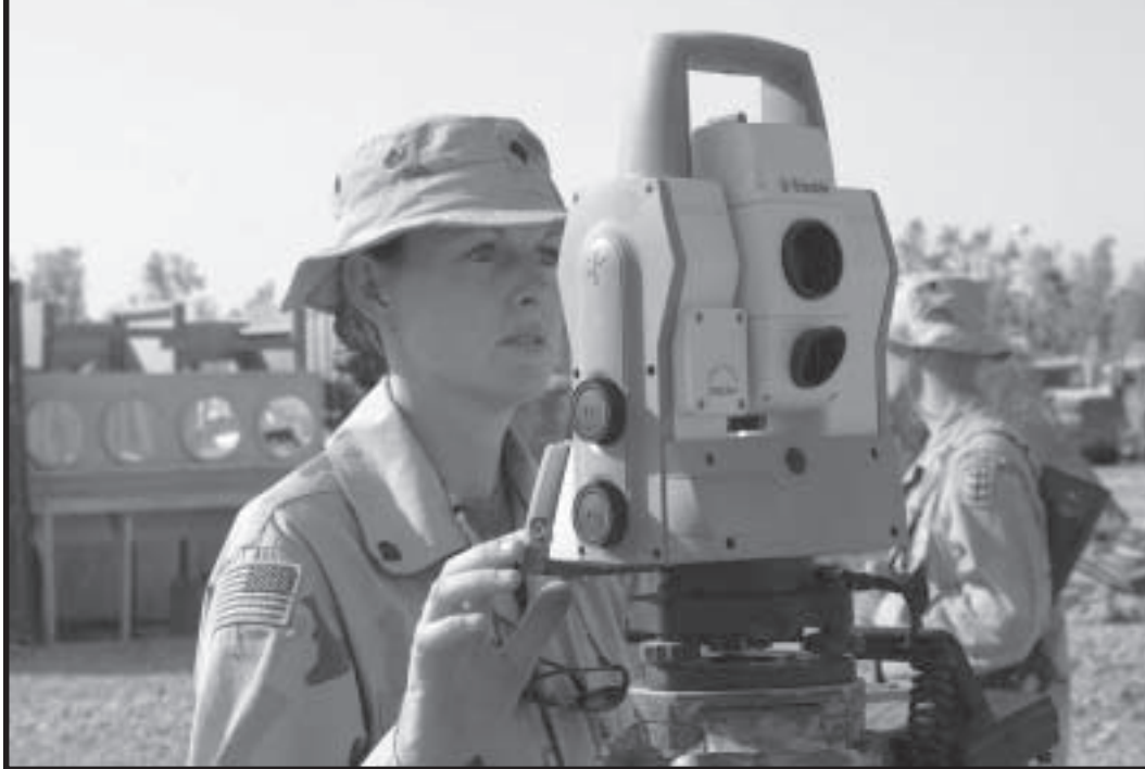
A soldier from the 320th Engineer Company (Corps) (Topographic) uses an automated integrated survey instrument at LSA Anaconda.
