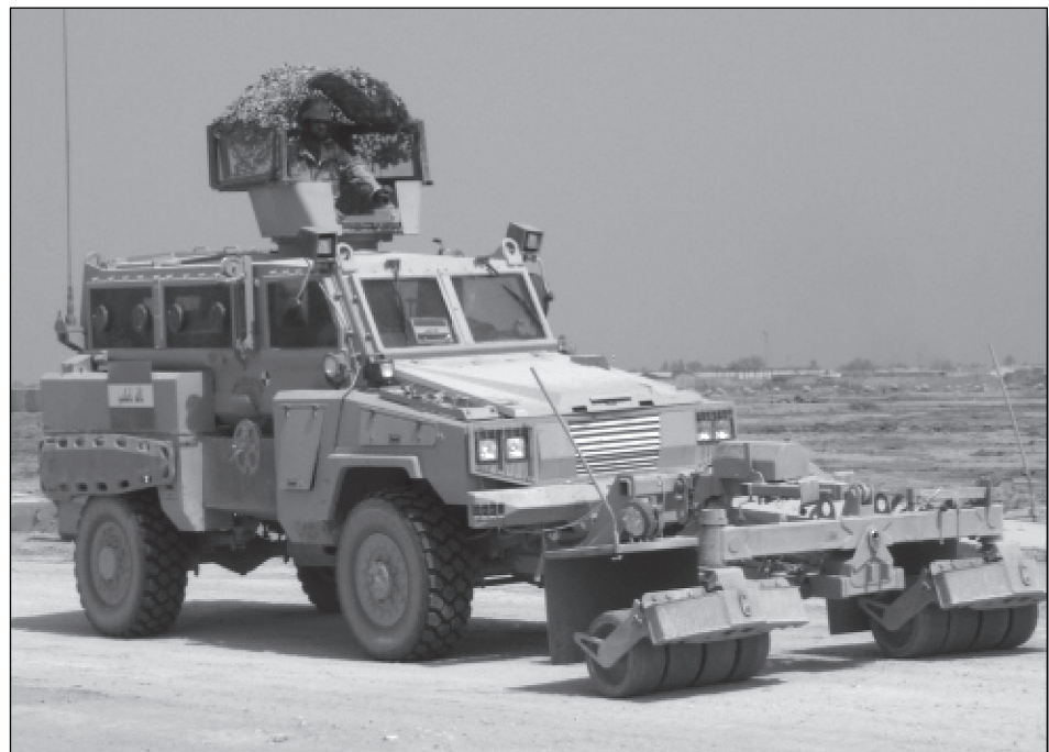
Iraqi Soldiers conduct a mock patrol in an RG-31 MK III with SPARK.
