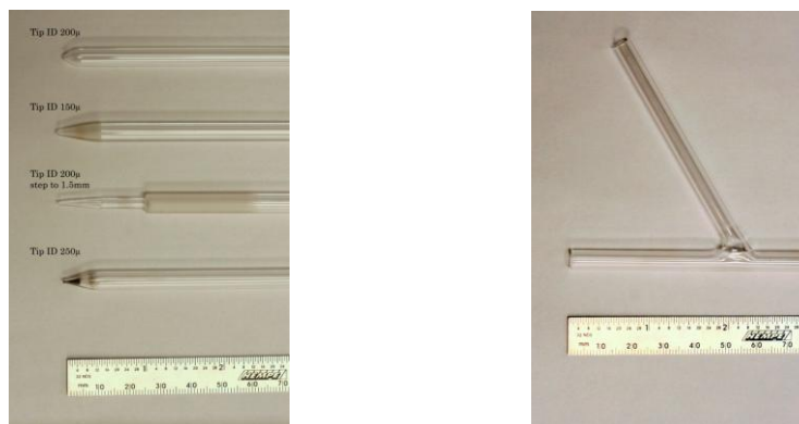
Figure 3.1.1 : The design iterations of the quartz sampling probe and the Y- Section
