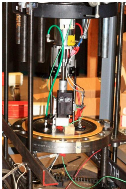
Figure 2.3: The riser section under the table with the base flange
