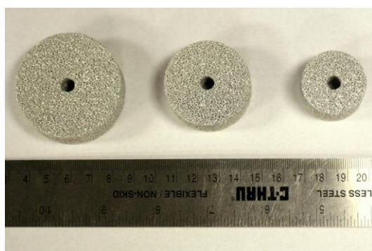
Figure 2.6: Metal foams with 100 ppi and diameters 50 mm, 40 mm and 25 mm
