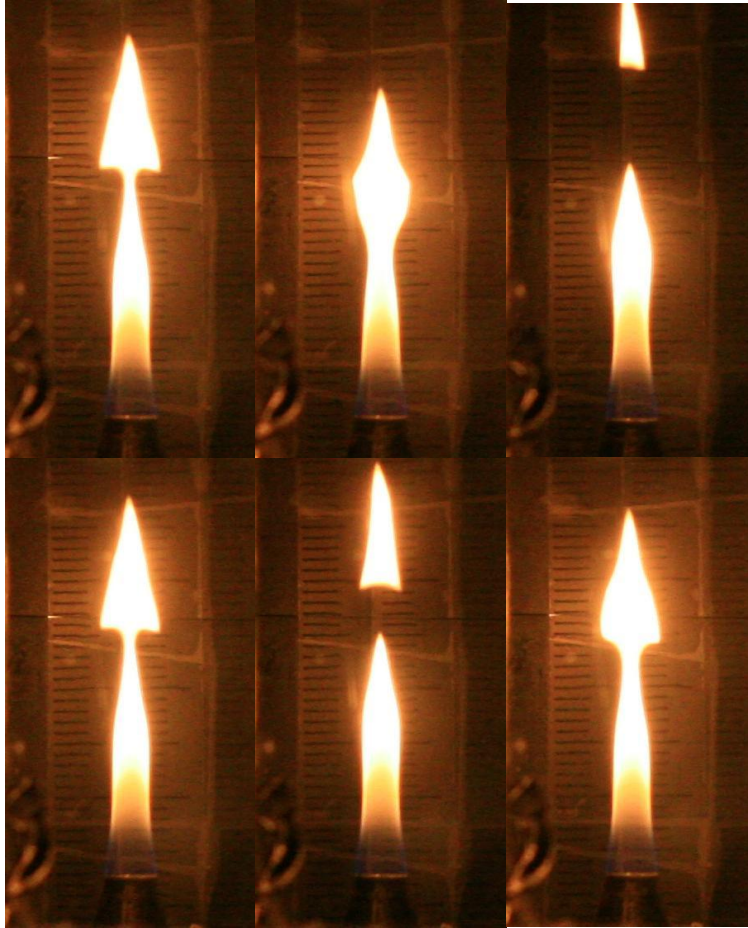
Figure 2.9: The sequence of images clockwise from left shows effects of buoyancy induced instabilities at 12 atm
