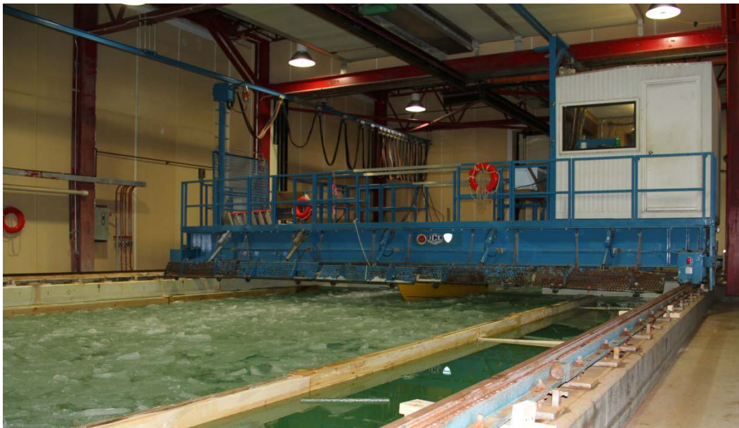
Figure 1. Picture of front view of boat attached to carriage; right side of carriage is the instrumentation cabin.
