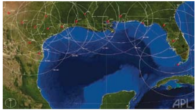
Lincoln Laboratory is supporting the FAA's development of ADS-B surveillance applications over the Gulf of Mexico. Satellite-derived positions for ADS-B will be merged with ground radar tracks to provide a high-quality integrated surveillance picture to air traffic controllers.
