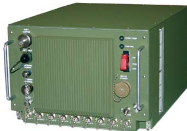
Lincoln Laboratory developed and successfully tested this multichannel signals intelligence receiver, which has enabled the Laboratory to rapidly innovate, develop, and test novel sensor capabilities for a variety of critical national problems. Key features include low noise figure, wide bandwidth, and direction-finding capability.
