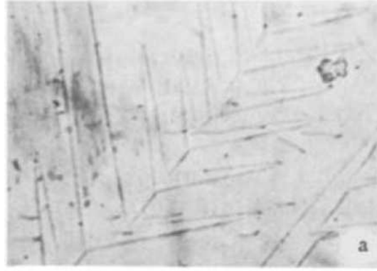
Figure 3.5: Fir tree magnetic domain pattern in (100) Fe-Al that is slightly mis-oriented [81].
