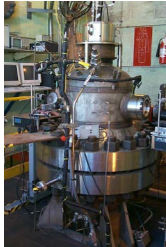
High Pressure Chamber (125 Bar) with Optical Access
