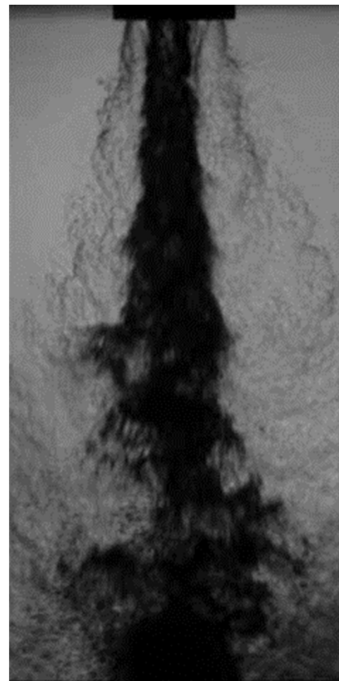
Back-lit Imaging Coaxial LN 2 -GHe Jet p_c = 400 psia
