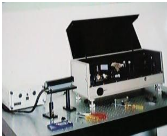
Fig.45 Optically pumped tunable laser based on a LiF crystal with F_2^+ color centers
