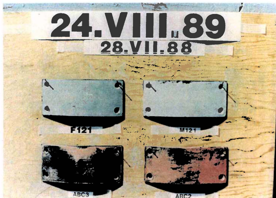
Figure 7. After 1 year of dynamic/static exposure, ABC3 completely lost one layer (red) of AF coating. ABC2 shows similar erosion. Loss of green AF coating appeared on the middle of the edge of M121.
