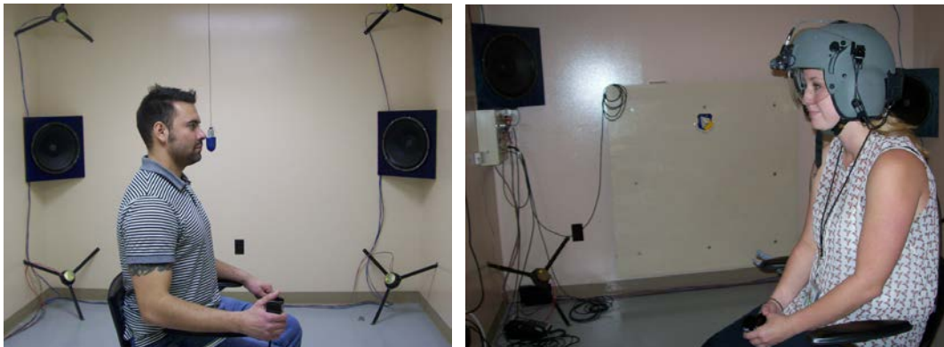
Figure 4. Subjects in REAT facility with and without the HGU-56/P flight helmet
