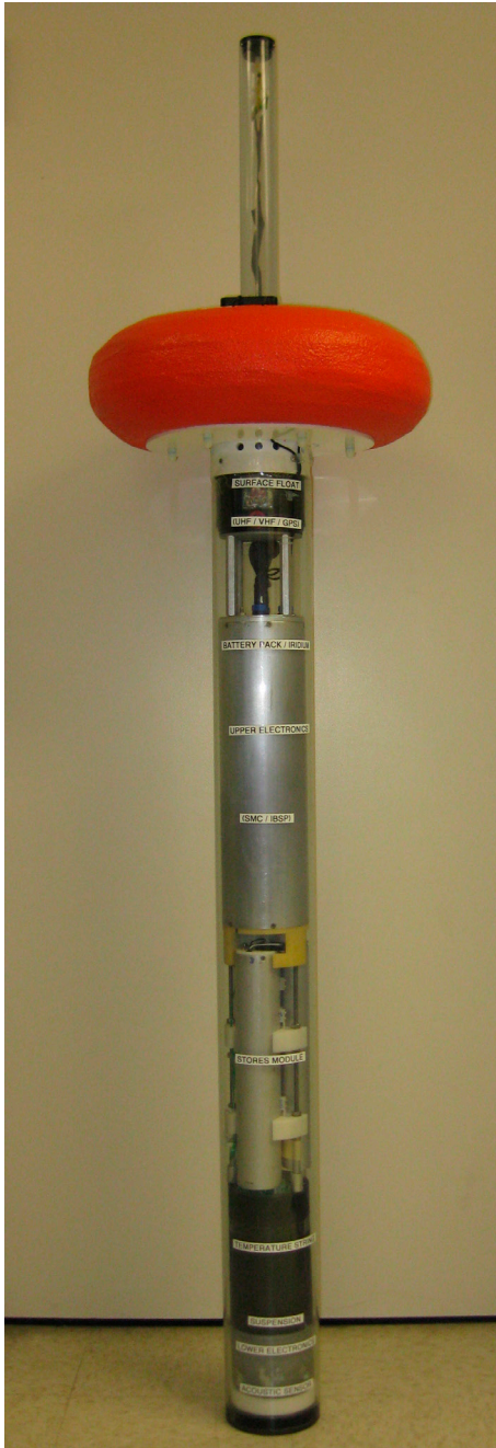
Fig. A-1 – SEA Buoy in Clear Canister with Test Surface Float
