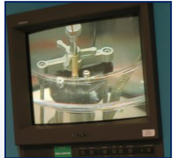
Thermocouple lid designed by Resodyn Acoustic Mixers, Inc.
