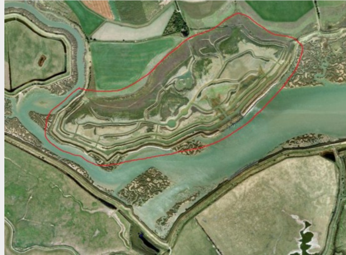
Engineered dendritic ditches in managed realignment site, UK
