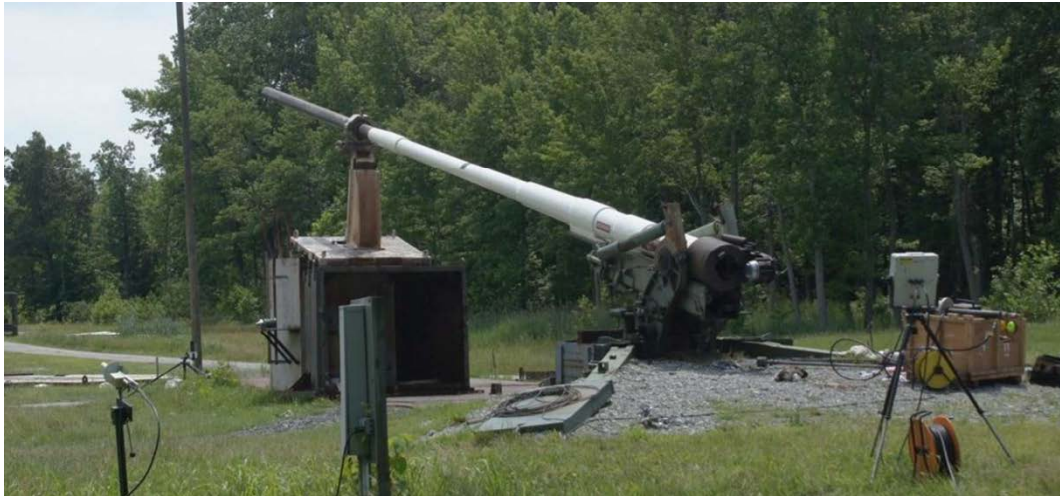
Figure 25. 178-mm HARP gun and experimental setup.
