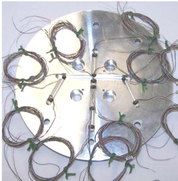
Figure 19. All 10 pressure sensors installed into the transducer section.
