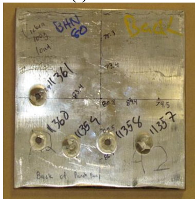
Figure 20. Photographs of (a) ECAE-processed 6- × 6- × 1/2-in AZ31B plate. Photos of the ballistic tested samples are given in (b) as received, (c) texture A, and (d) texture C conditions. The top row of photos is the front of the plate and the bottom row is the back of the plate.
