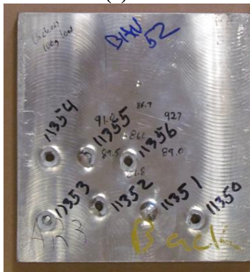
Figure 20. Photographs of (a) ECAE-processed 6- × 6- × 1/2-in AZ31B plate. Photos of the ballistic tested samples are given in (b) as received, (c) texture A, and (d) texture C conditions. The top row of photos is the front of the plate and the bottom row is the back of the plate.
