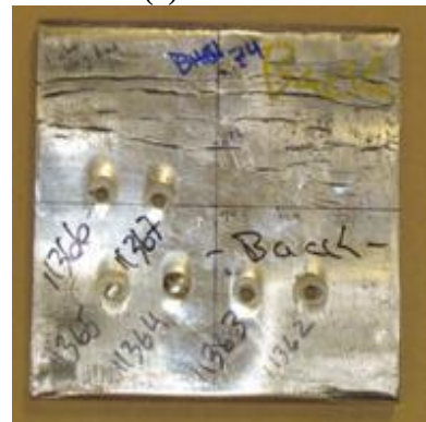
Figure 20. Photographs of (a) ECAE-processed 6- × 6- × 1/2-in AZ31B plate. Photos of the ballistic tested samples are given in (b) as received, (c) texture A, and (d) texture C conditions. The top row of photos is the front of the plate and the bottom row is the back of the plate.
