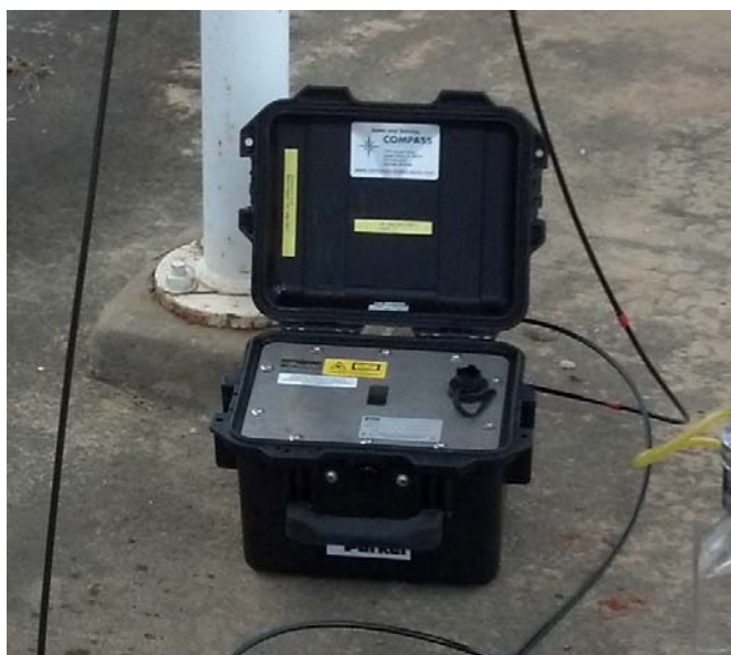
Figure 3. Parker IcountOS light obscuration particle counters utilized for evaluation.
