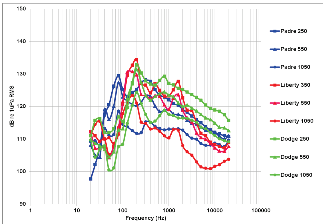
Figure 8. One-third octave analysis results at selected distances for dredges in transit to pump-out stations.
