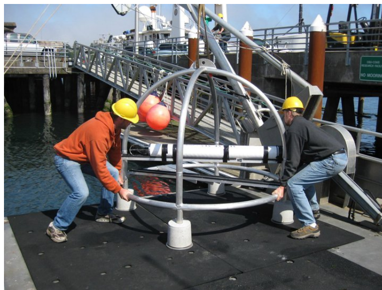
Figure 2. Configuration of a passive acoustic sensor within its mooring frame. See Figure 1 for the distribution of four of these sensors across the study area.
