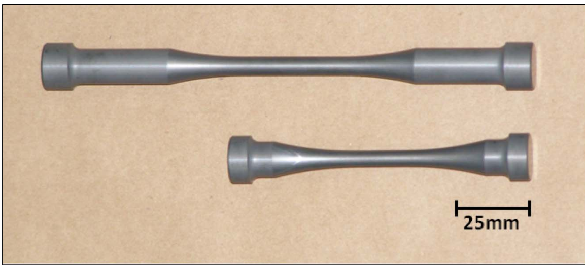
Figure 3. SiC-N uniaxial tension specimen configurations.
