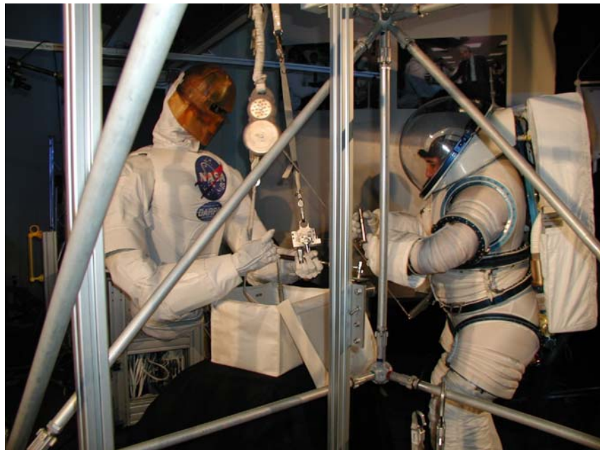
Fig 2. Robonaut working with Astronaut Nancy Currie in a prototype Advanced Space Suit
