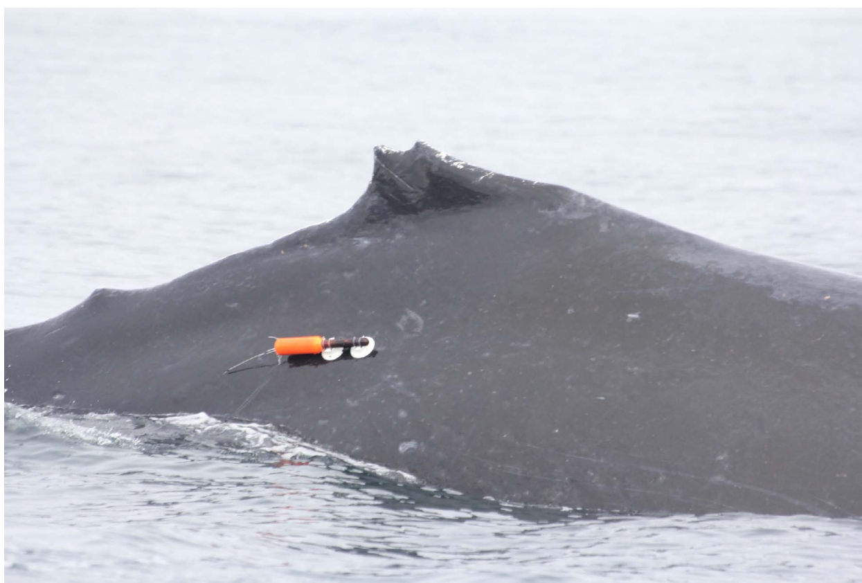
Figure 2. Photograph of an Acousonde™ 3A acoustic recording tag attached with suction cups to a humpback whale (photo by Bree Witteveen, University of Alaska (Fairbanks), NMFS Scientific Research Permit No. 14296)
