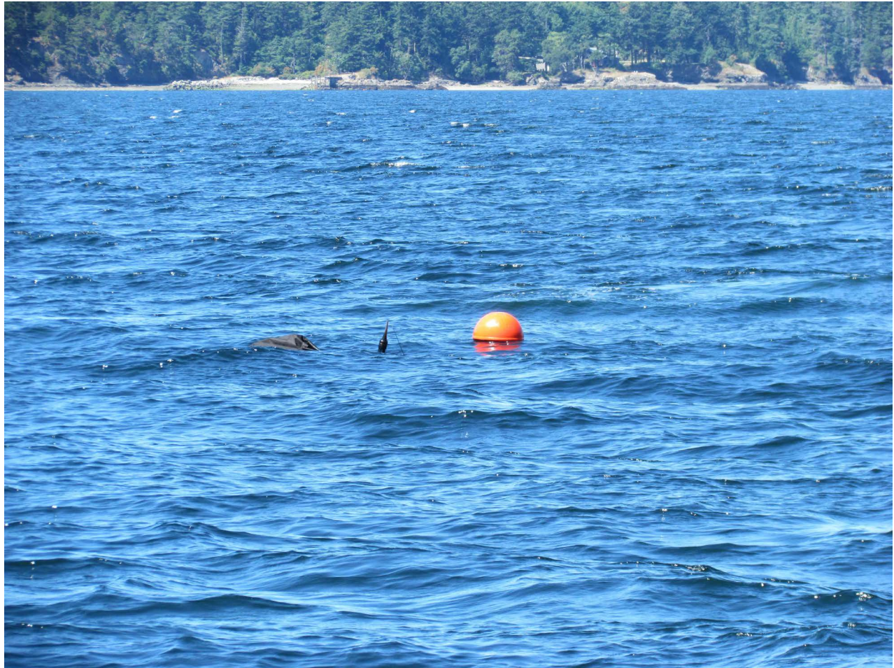
Figure 2 Surface drifter (SVP Microstar, http://www.pacificgyre.com ) just after deployment at Station 5 on August 2 nd 2011. Black drogue is still visible at the surface. The orange surface sphere contains a GPS unit that is remotely tracked and provides position information at 10 minute intervals.
