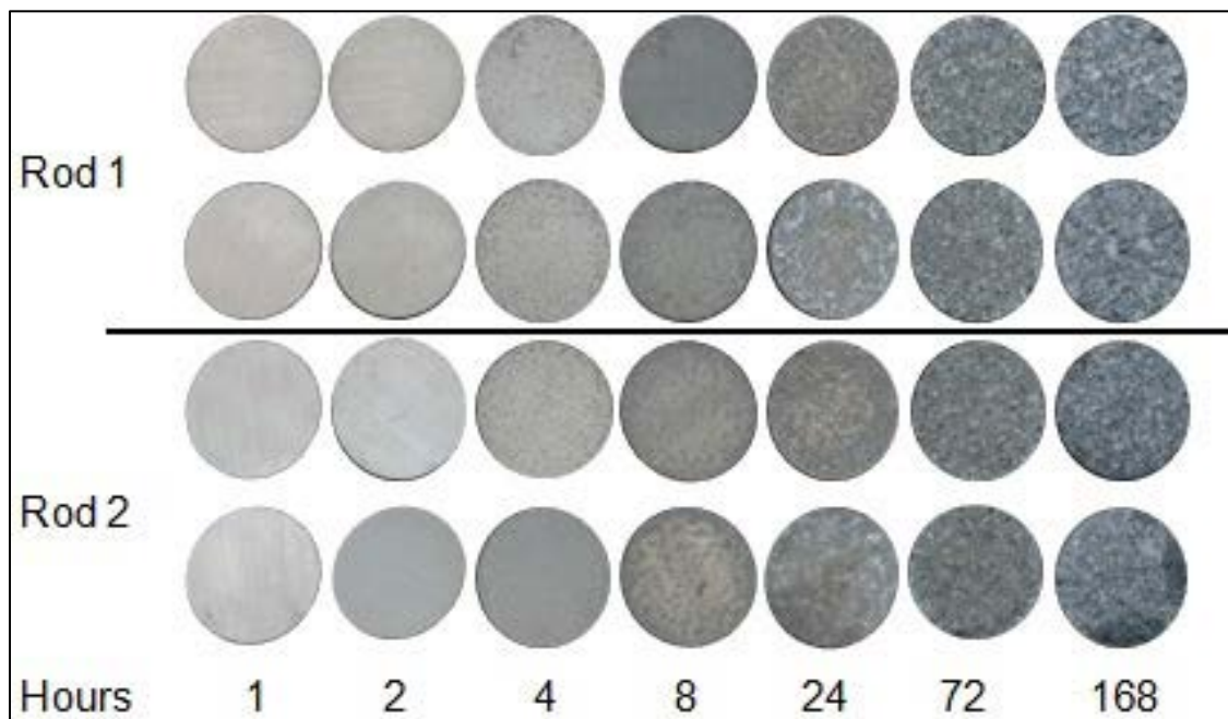
Figure 9. Optical photographs detailing changes in surface appearance after the indicated number of hours for the Fuji Light samples subjected to the salt fog test chamber.
