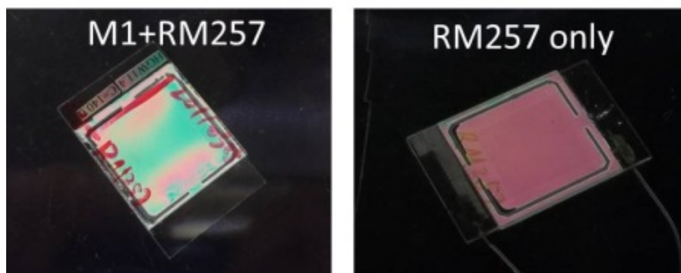
Fig. 9 Photographs of two PNLCs containing different types of monomers.
