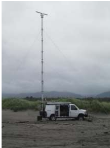
Figure 2. SIO RadarVan operating at the Clatsop Spit, South Jetty, Ft. Stevens State Park, OR
