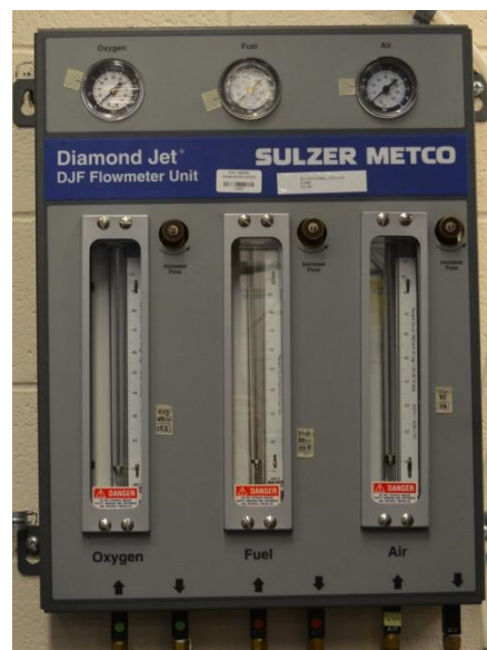
Figure 13 - DJF Flowmeter Unit Used To Control Spray Gun
