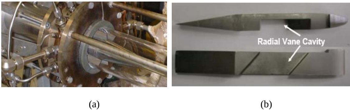
Figure 2.4. a) Photograph of radial vanes housed in UCC and b) Radial Vane Cavity machined out of straight vane [10].
