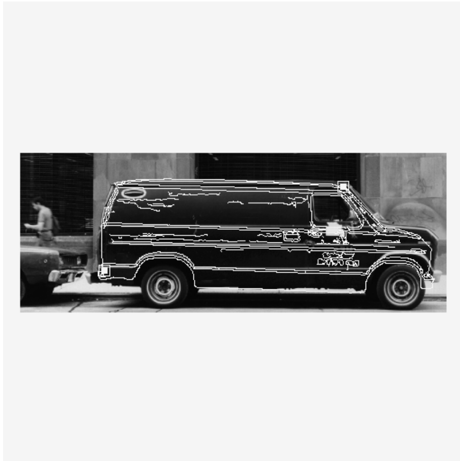
Figure 8.14 The Ford Econoline 150 test input with the retrieved model overlaid on it. The recovered transformation (rotation, translation and scaling) was based solely on the basis pair, and not on a best least-squares match of all corresponding feature pairs.
