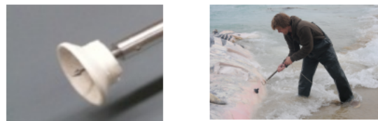
Figure 2. Flexible latex suction cup built by Cetacean Research Corp. and modified with a 0.64 cm barb with conical pointed barb (left image), and field testing vertical holding strength of a suction cup (type I) tag with barb on a stranded humpback whale (right image).
