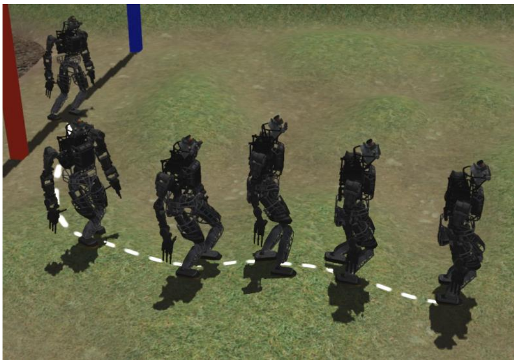
FIGURE 3.4.1: Hill crossing using dynamic foot-placement walk (DFPW). The robot is able to walk slowly by stepping on specific locations where the robot can remain stable.
