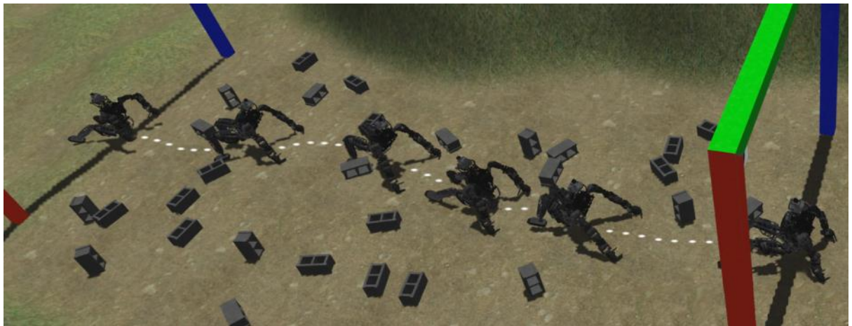
FIGURE 3.4.4: Debris crossing using pentad-walk (PW, see movie ). The robot crosses the hill section autonomously, walking towards the center of the next gate. The robot is able to recover from tipping in any direction and can locally modify its path if it gets stuck.
