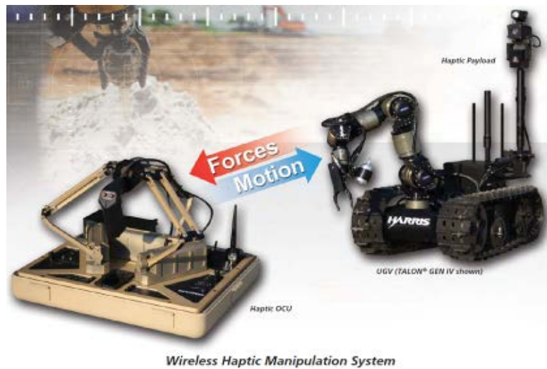
Figure 5. The haptic manipulator used with stereovision for the Talon robot experiment.
