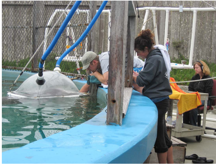
Figure 1. Photograph taken during an experimental session showing the equipment set-up which includes the metabolic hood, the dolphin stationed under the metabolic hood, the acoustic recording equipment and operator, the dolphin trainer, and the assistant taking notes and recording respirations.
