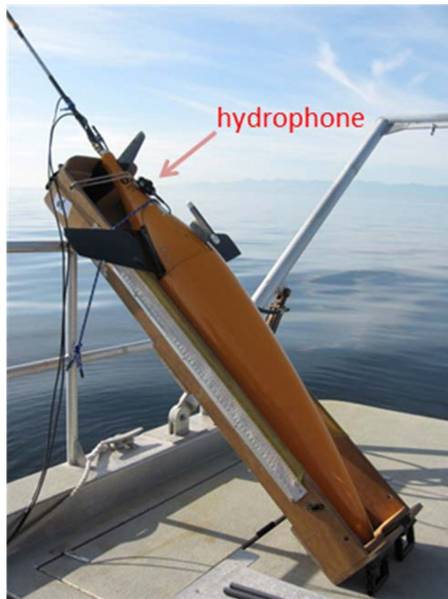
Fig. 1. A Seaglider™ equipped for passive acoustics
