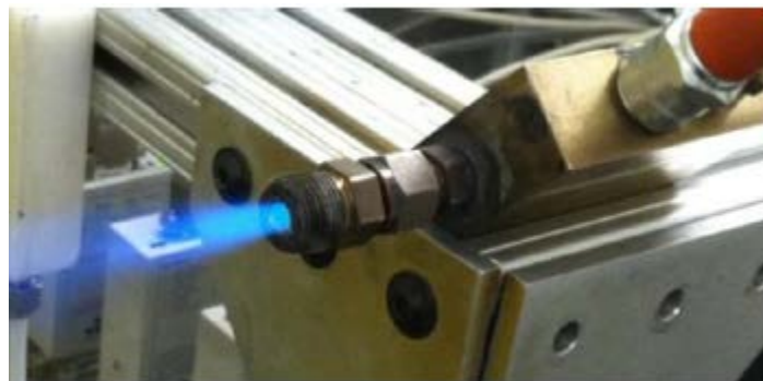
Figure 32: Ethylene-air ignition torch.
