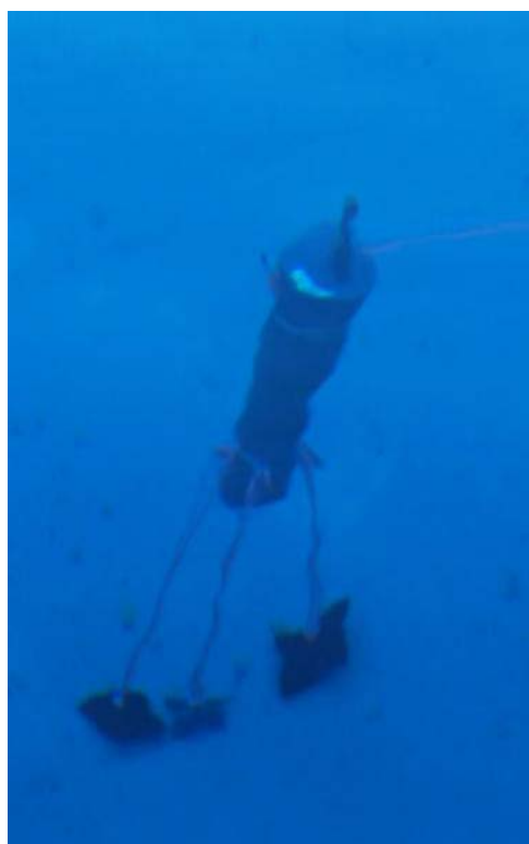
Figure 1. a) Photograph of the DSG deployed at the bottom of the beluga exhibit at the Mystic Aquarium and b) spectrogram sample of beluga whale calls recorded with the DSG.
