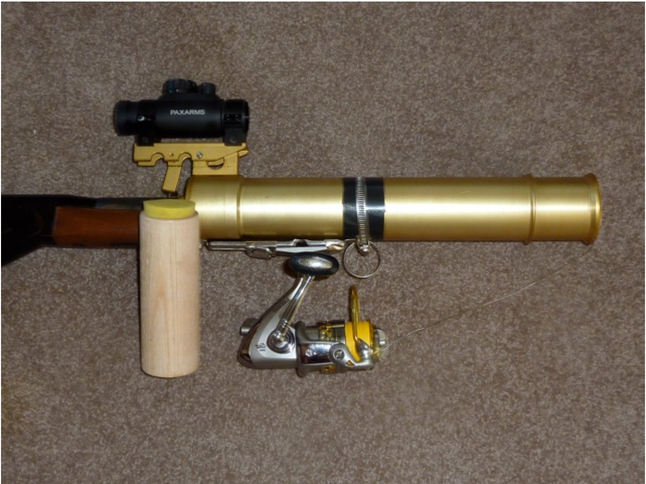
Figure 4 Prototype of rifle, Paxarms Remote Delivery System (PRDS) that will be used to implant the oximeter probe into the muscle. The PRDS consist of a rifle with a laser scope and a guideline.
