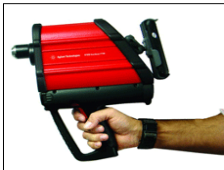
Figure 3.3: Image of Agilent Exoscan 4100 used for FTIR spectra collection[32].
