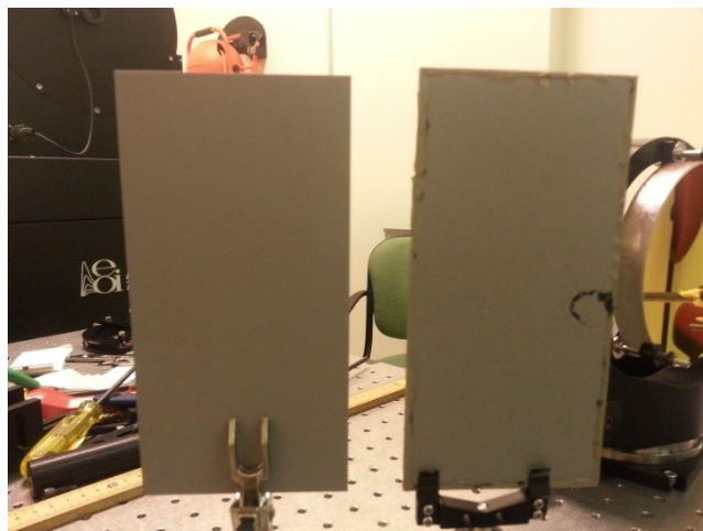
Figure 3.12: Picture of the scene shown in the hyperspectral image in figure 3.13. The sample on the left is the untreated sample and the one on the right was treated to the level of visible degradation. Both samples are from sample set A. An exposed blister can be seen on the right-center of the treated sample.
