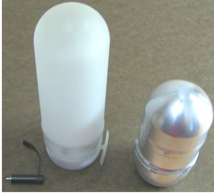
Figure 4. Image of motor with rotating wing concept and prototype 40-mm projectile.
